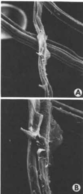
Figure 6. Scanning electron micrographs of a delaminated zinc chloride-bonded rayon nonwoven (A—128 \times , B—425 \times )
